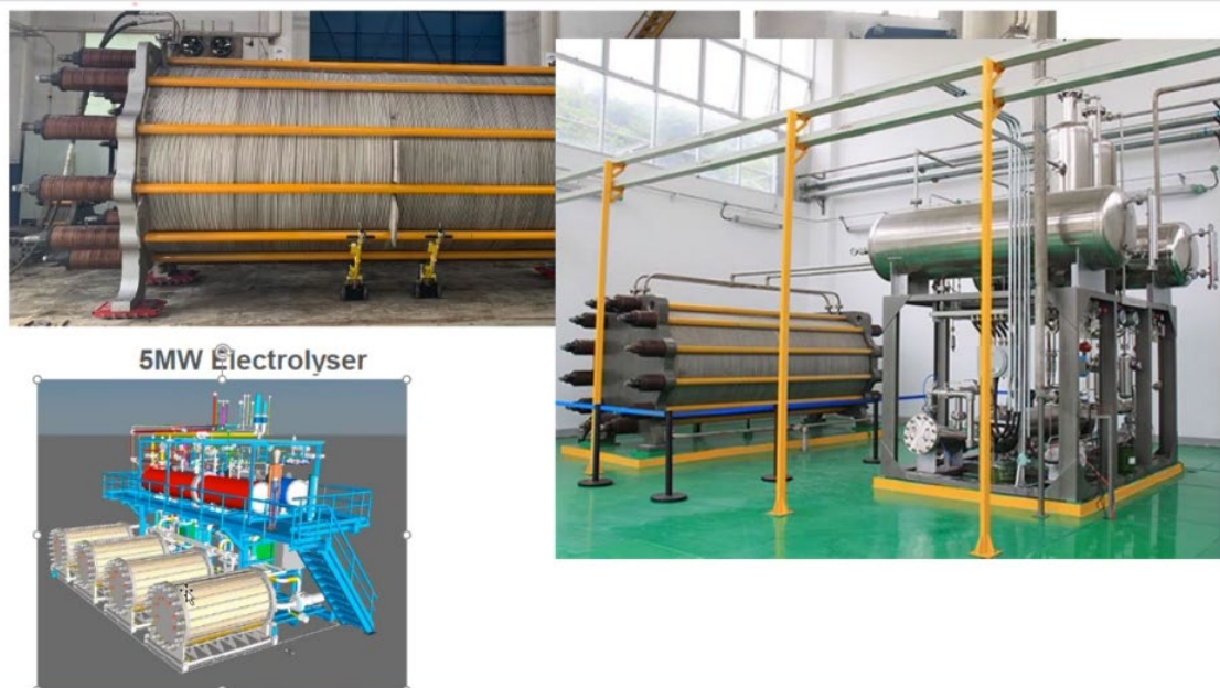
Figure 2-4 5 MW Electrolyser Packages (Ref. open-source data)
